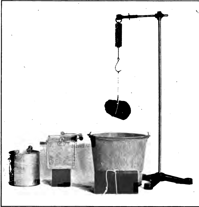
FIG. 10. Apparatus used to illustrate the law of Archimedes.
